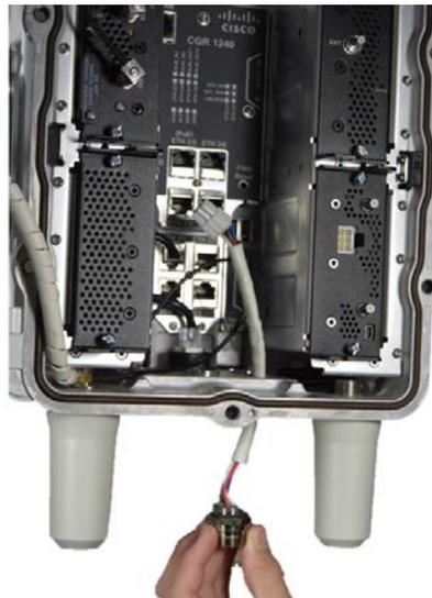
9. Insert the PLC Signal Cable into the 6-Pin connector, see item 1, on the front of the CAM3S/CAM3M.
