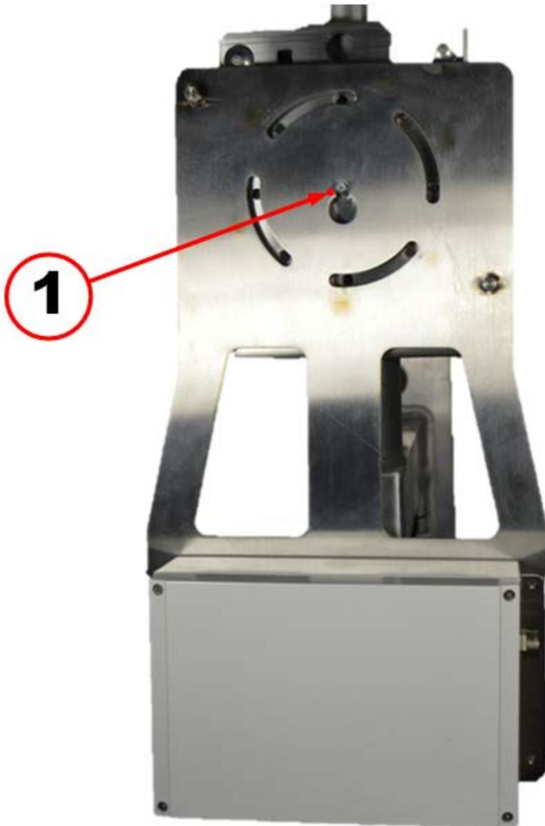
5. Position the CGR Mounting Bracket over the center stud with self-locking hex nut, see item 3, and slide down behind hex nut.
