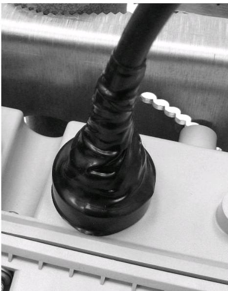
3. Ensure that the tape fully covers the cable strain relief.
