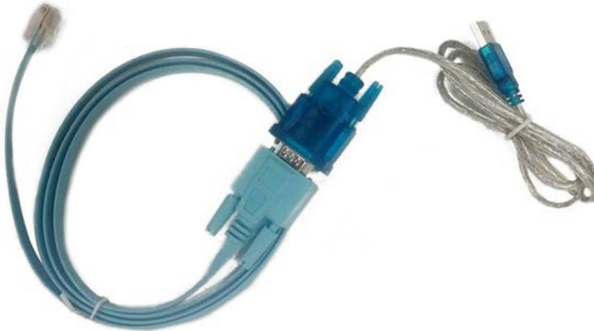
4. Plug the blue Cisco DB9-RJ45 Serial Cable, RJ45 end, into the CGR's RJ45 Connector, see figure, that you accessed located on the right hand side top of the CGR.
