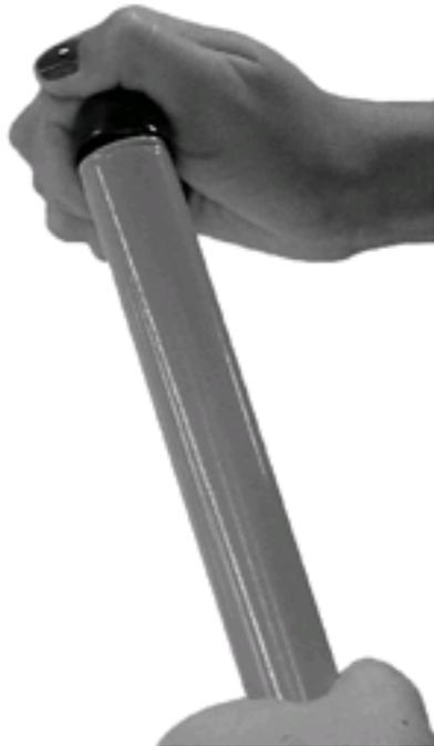
2. Slide the silicone seal over the base of the remote antenna.
